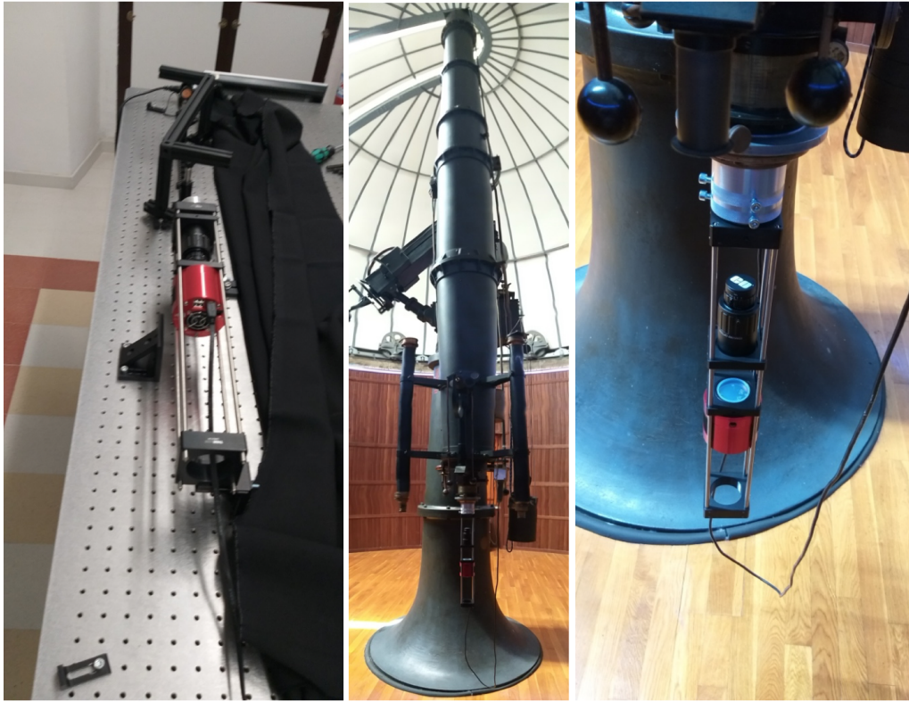
Fig. 4. The CMOS camera mounted on the optical bench for preliminary laboratory tests, in Teramo; and CMOS camera mounted on the focal plane of the Cooke Telescope for the acquisition of astronomical images of Mars and Jupiter. The optical adapter is placed between the camera and the focal plane to test different magnifications.
