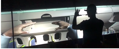
Fig. 2. User interacting with an airplane overhead bin in a virtual environment, simulation conducted in the framework of CASTLE Project. The user is immersed in a digital model of an airplane and its experience is being displayed on the CAVE (Cave Automatic Virtual Environment). Courtesy: Virtual Reality and Simulation Laboratory (VLAB).
