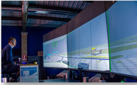
Fig. 1. Virtual Reality simulation of Airport Control Tower operations in the realm of RETINA Project conducted in the premises of the University of Bologna, Forlì campus. A digital model of Bologna's airport is displayed on the CAVE (Cave Automatic Virtual Environment) for an immersive simulation for the Air Traffic Operator. Courtesy: Virtual Reality and Simulation Laboratory (VLAB).
