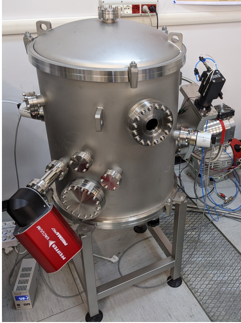
Fig. 3. CAPSULA Thermal Vacuum Chamber. The Mass Spectrometer (red block containing the electronics) is visible.
