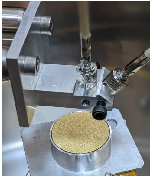
Fig. 7. UHV Infragold realized for IR reference measurement in vacuum.
