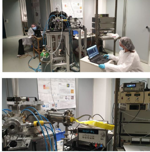
Fig. 6. Calibration activities: on the top panel the spectrograph prototype with the EUV CCD camera during spectral calibration; on the bottom panel the MIRA-MCP detector demo integrated on the spectrograph prototype.
