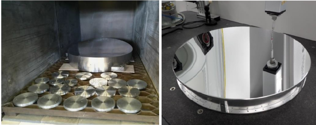
Fig. 5. On the left is the image of the PTM together with 150 mm diameter samples inside an oven to carry out a hot thermal treatment, and on the right is the image of the 0.7 m diameter BreadBoard mirror after having carried out a diamond turning.
