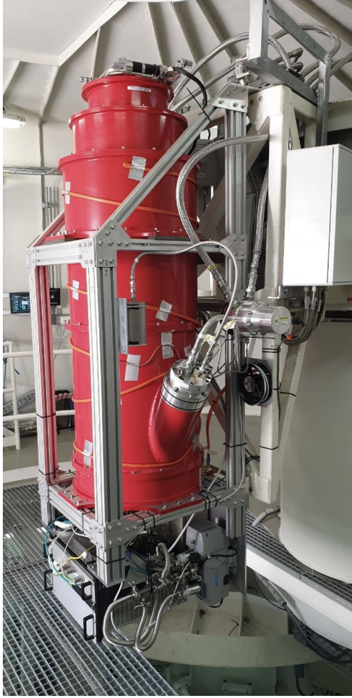
Fig. 1. MISTRAL in its final position on the SRT turret structure, a rotating structure that carries several instruments and allows observers to position them at the Gregorian focus one at a time. Credits: M. Murgia, INAF-OAC.
