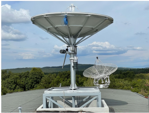
Fig. 10. The new solar radio polarimeter (TSRS 2.0) at the Basovizza Observing Station in Trieste is visible in the foreground, and the older solar radio polarimeter (TSRS 1.0) in the background.
