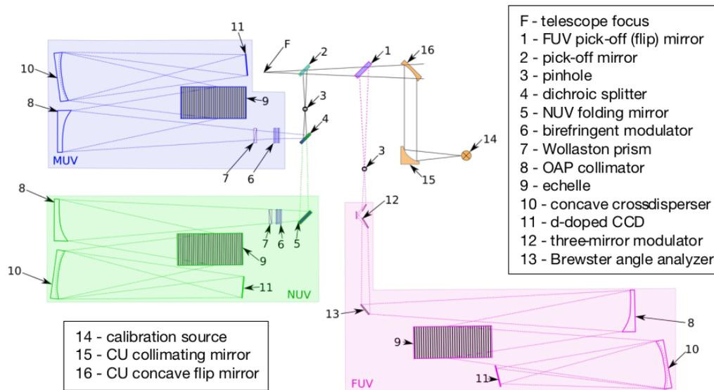
**Fig. 1.** Design of Pollux for LUVOIR-A, showing the 3 UV channels. Taken from The LUVOIR Team (2019).
