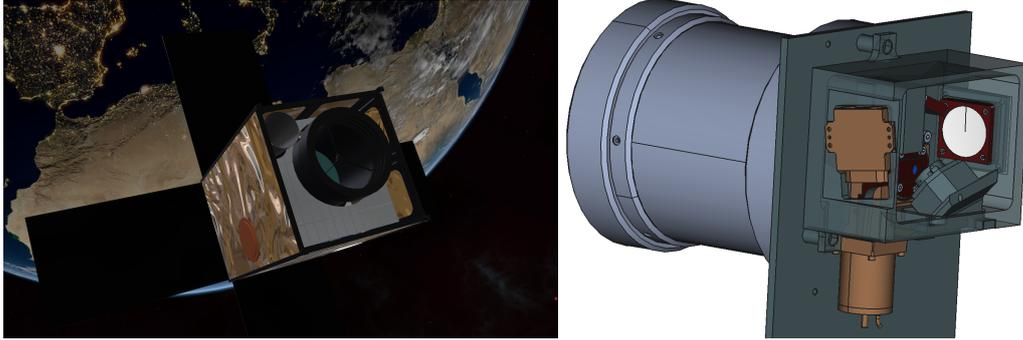
**Fig. 4.** Left: the CASSTOR nanosatellite. Right: view of its 12-cm telescope and payload.
