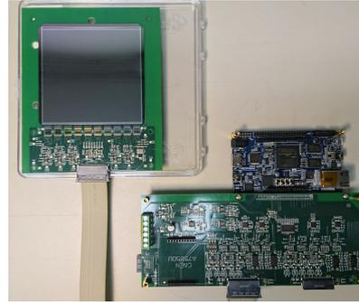
**Fig. 9.** Single silicon sensor and its readout: from bottom to top the ADC board, the DE10-Nano board, and one hybrid board with ten IDE1140 FE ASIC's and one sensor.
