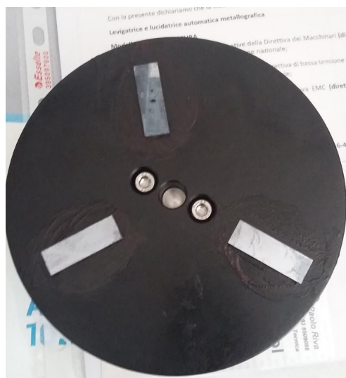
Fig. 2. Top view of the rotational head of the lapping machine through which three crystals can be machined at once. The floating head allows to impress the same strength over the three crystals therefore the same curvature radius is achieved for the three sample with few percent of uncertainty.
