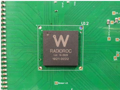
**Fig. 3.** Picture of the RADIOROC, used for the measurement, mounted on an evaluation board provided by Weero.
