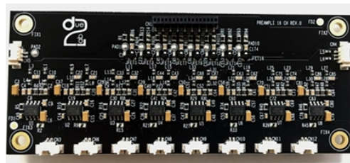
Fig. 3: The 16 channel CSP. Each surface of the hybrid board contains 8 CSP readout channels.
