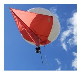
Fig. 1. Skyhook tethered Helikite.
