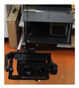
**Fig. 2.** Gimbal that hosts a HD VIS camera and an IR camera for night vision.
