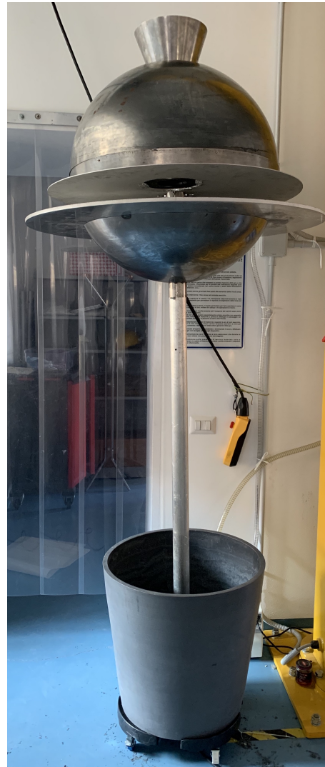
Fig. 2. Picture of the whole system, including the pole, the vase and the base with wheels.
