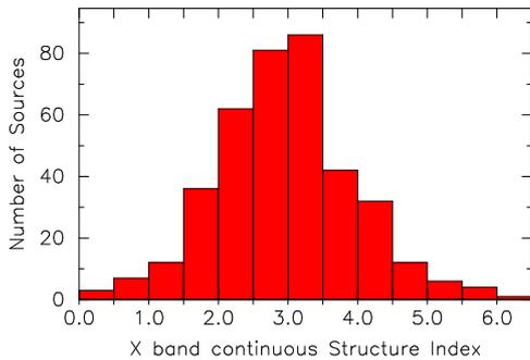
**Fig. 4.** Distribution of the 8.4 GHz structure index for the ICRF2 sources that have an optical counterpart brighter than magnitude 18 in the LQAC and with a structure index available. Sources with a structure index less than 3 are suitable for the alignment with the Gaia frame.
